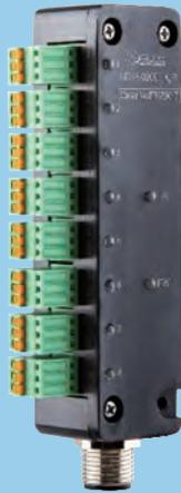
Mini Hub is the most compact IP20 hub in IO-Link solutions. It adopts a standard M12 A-code interface, which meets the IO Link V1.1.3 standard. It has 3 pluggable terminals for easy installation and maintenance. 8DI and 4DI/4DIO, making it particularly suitable for small control cabinet, remote control cabinet, and other application with limited installation space.
